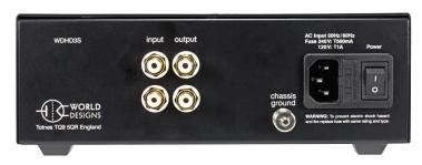
Rear panel layout is simple with clearly-labelled and reasonably wellspaced RCA sockets for the signal input and output.
