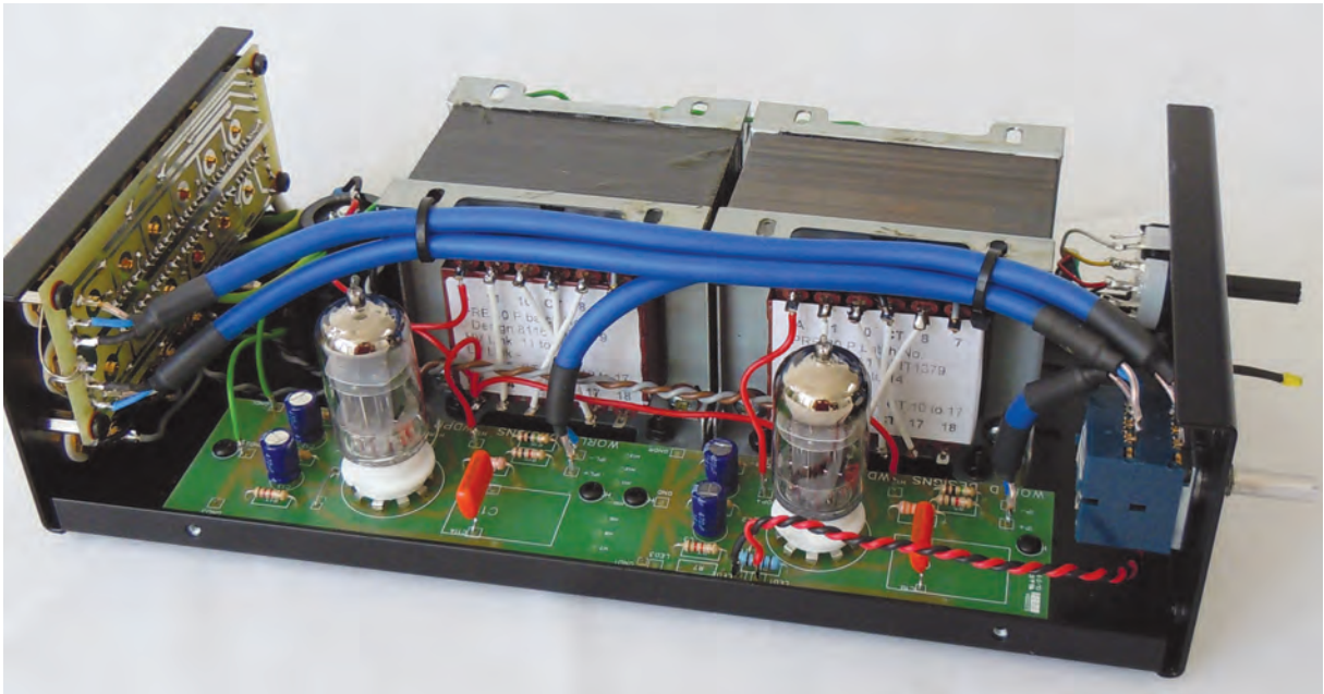
Fig. 15 Signal Wiring and LED
